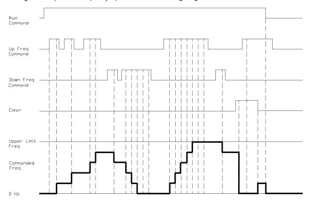
Figure 29. Up/Down Frequency Operation Control Timing Diagram.
