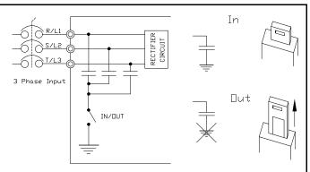
Figure 5. The **Grounding Capacitor Switch** is used on typeforms **230-volt**15 HP to 20 HP and the 40 HP to
