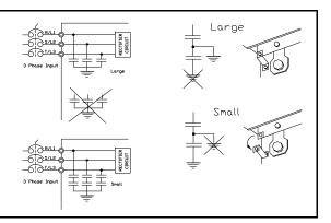
Figure 7. The **Grounding Capacitor Screw** is used on typeforms **460-volt**175 HP and above.
