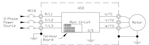
Figure 3. G9 ASD/Motor Typical Connection Diagram.
