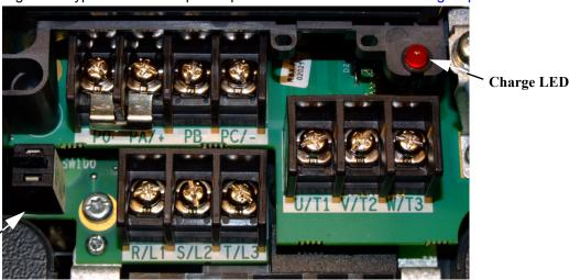
Grounding Capacitor Switch — Pull for Small capacitance/push for Large capacitance.
