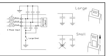
Figure 6. The **Grounding Capacitor Bar** is used on typeforms **230-volt** 75
