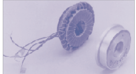
Fig 13 - axial airgap motor, wound stator core and diecast rotor core
